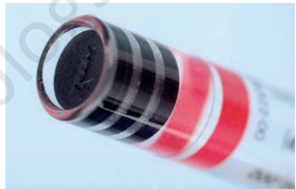
Figure 7-3. Silicone rubber plunger is slightly indented from the rim of the glass.
