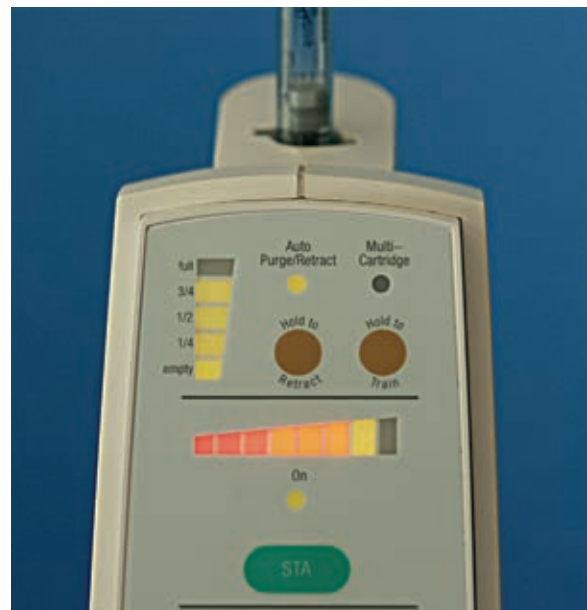
Figure 20-16. Dynamic pressure-sensing (DPS) technology that provides continuous real-time injection feedback and identification of specific patient tissues has been shown to enhance the predictability of the periodontal ligament (PDL) injection. (Photo courtesy Milestone Scientific, Livingstone, NJ.)
