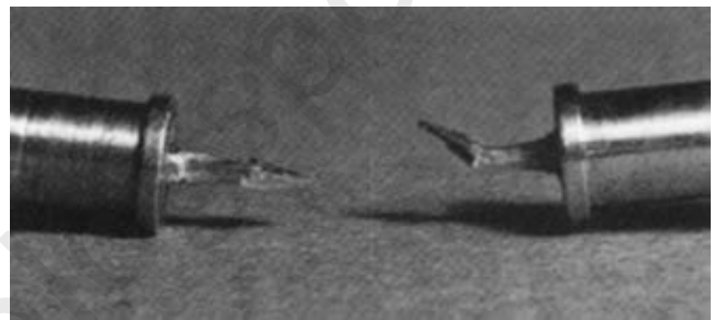
Figure 5-26. Note the bent harpoon of the syringe on the right.
